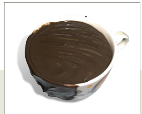
After filtration: retentate (filtration lees)
